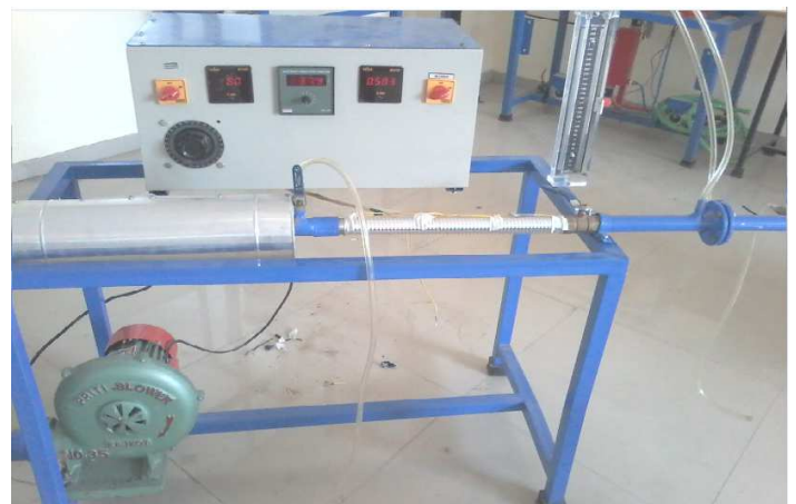
Fig. 1.Experiment set up of spiral fin tube heat exchanger
